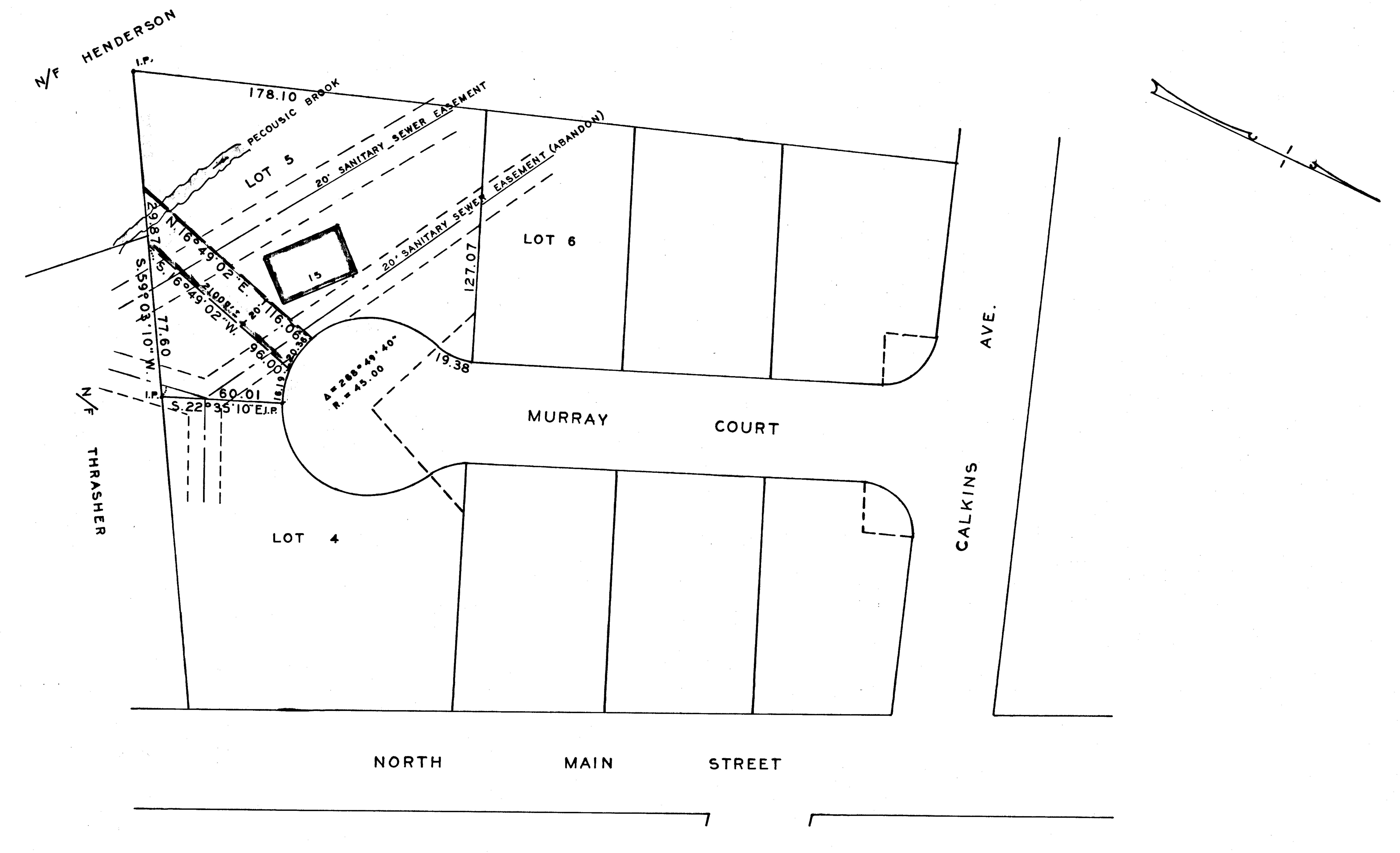
PLAN SHOWING 20' EASEMENT TO BE ACQUIRED FOR STORM DRAIN PURPOSES
