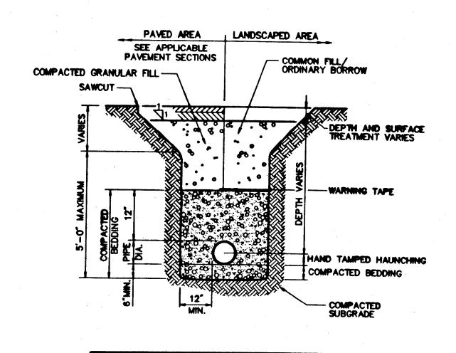
1. WHERE UTILITY TRENCHES ARE CONSTRUCTED THROUGH DETENTION BASIN BERMS OR OTHER SUCH SPECIAL SECTIONS, PLACE TRENCH BACKFILL WITH MATERIALS SIMILAR TO THE SPECIAL SECTION REQUIREMENTS.
