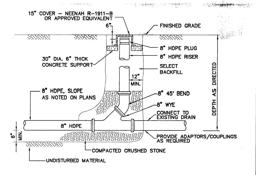
DRAIN LINE CLEANOUT DETAIL
