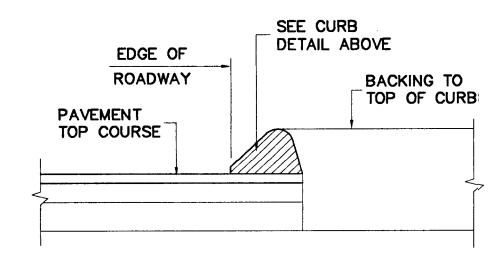
BITUMINOUS CONCRETE CURB
