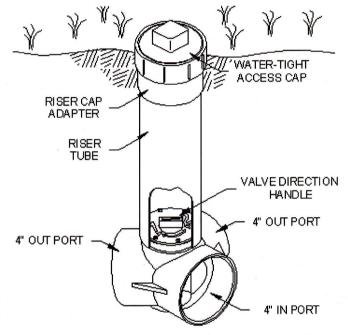
The Bull Run Valve is available in 4" sch 40 pvc and is suitable wherever septic disposal systems are used - in commercial, industrial, and residential applications.
